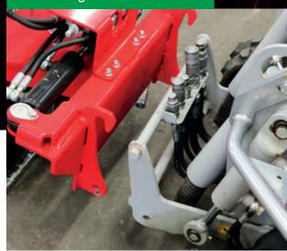
Lock the bracket. Remove hoses. Then it is easy to change attachments on the RC-1000. Everything is done in minutes, with no tools.
